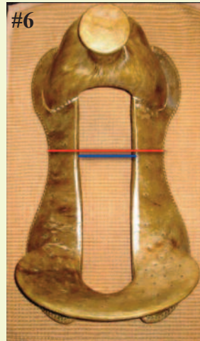
Red line is the outer most part of the twist, while the blue line is usually where the twist is measured.
