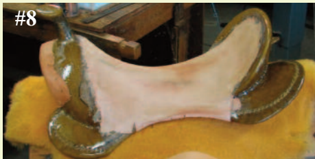
Ground seat under construction
