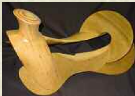
Excellent example of a custom made wade tree with wood post horn, awaiting rawhide covering. Note stirrup leather relief on the bottom of the tree.
