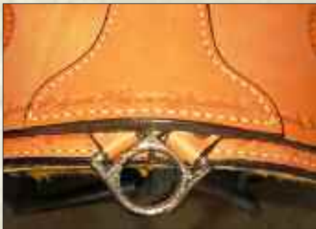
Cantle jockey installed so close to skirts, they interfere with the skirts' ability to flex at the rear corners.
